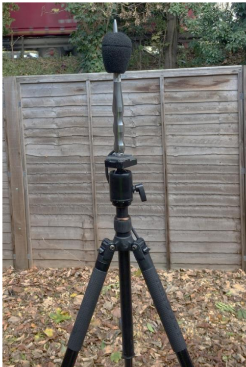
Plate 3.6 Typical noise monitoring equipment
